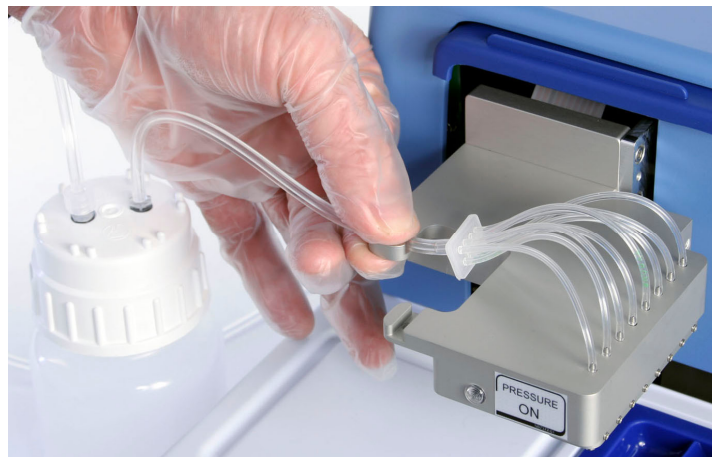
Figure 5–31. Replacing the tubing set and manifold
