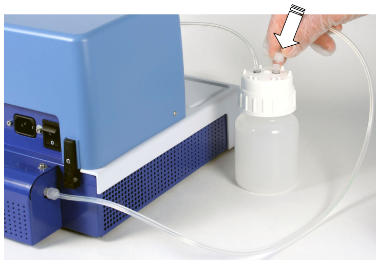
Figure 3-11. Connecting the hosing to the reagent reservoir
