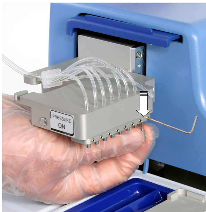
Figure 5–29. Pulling the dispensing valve downwards
