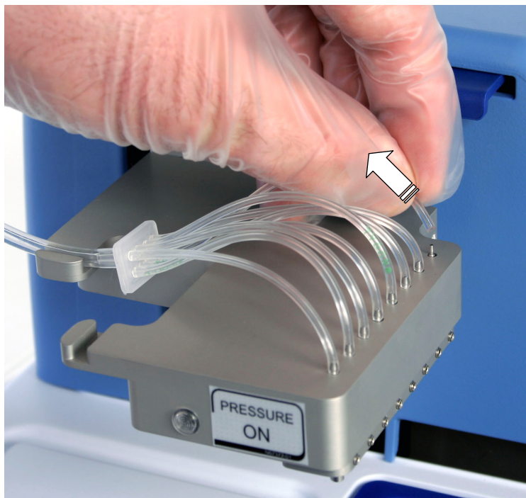
Figure 5–25. Detaching a dispensing valve tube end
