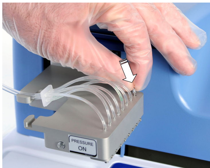
Figure 5–26. Reconnecting a dispensing valve tube end
