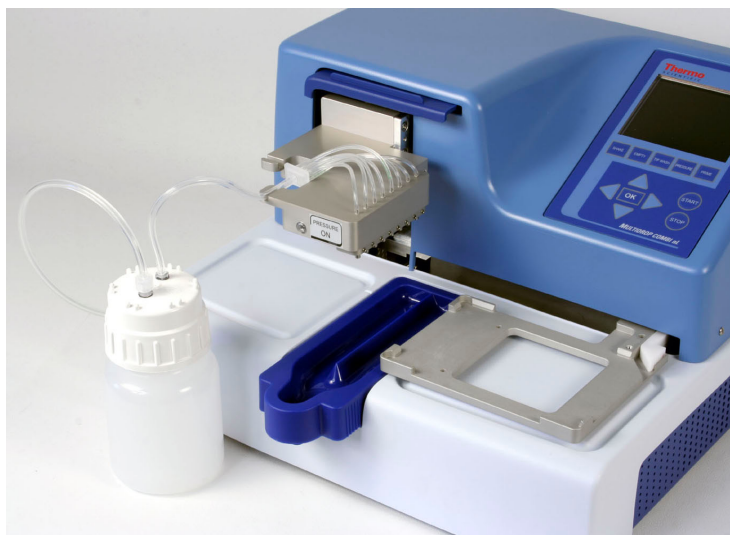
Figure 3–13. Reagent reservoir connected to the instrument
