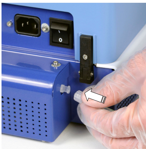
Figure 3–10. Connecting the hosing to the pressure/vacuum system
