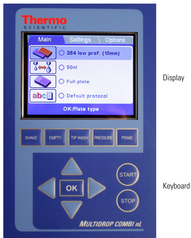
Figure 2–3. Close-up of the Multidrop Combi nL keyboard and display
