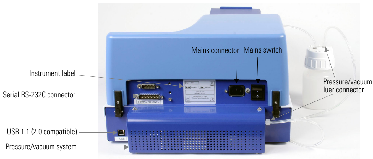
Figure 2–4. Multidrop Combi nL back view
