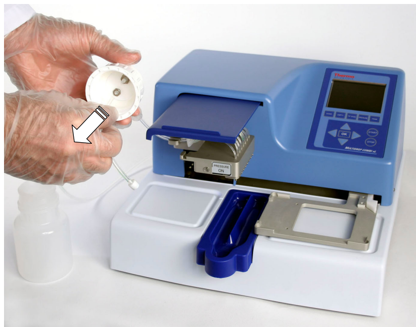
Figure 5–27. Removing the reagent filter with tube
