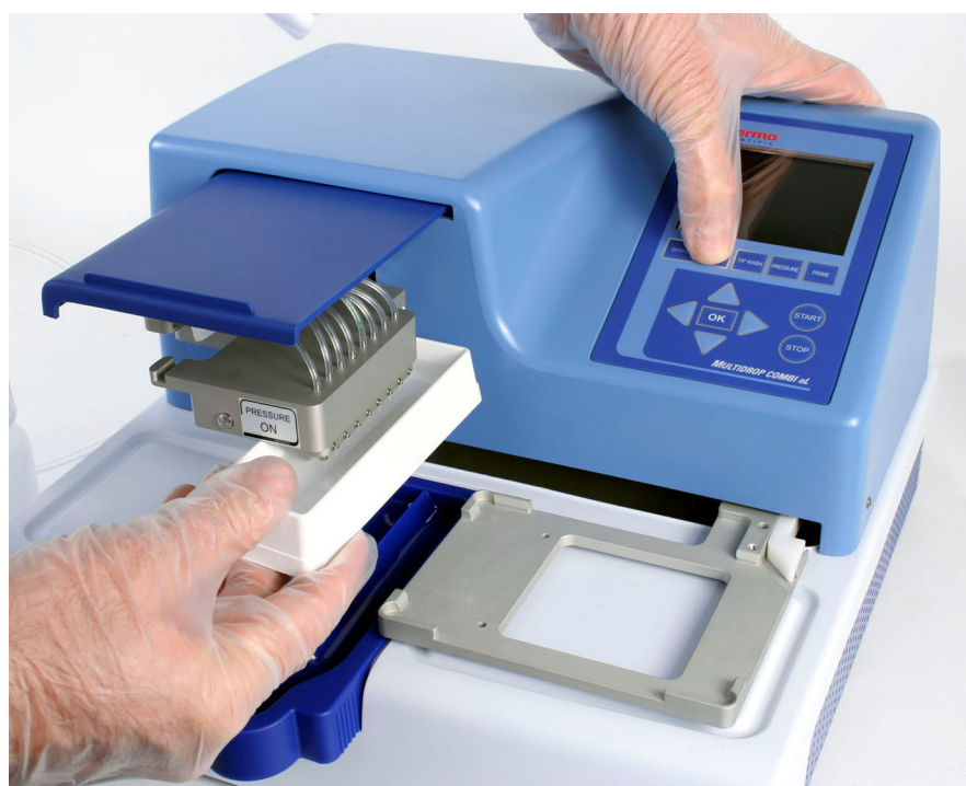
Figure 5-24. Cleaning the tubings using a reagent basin
