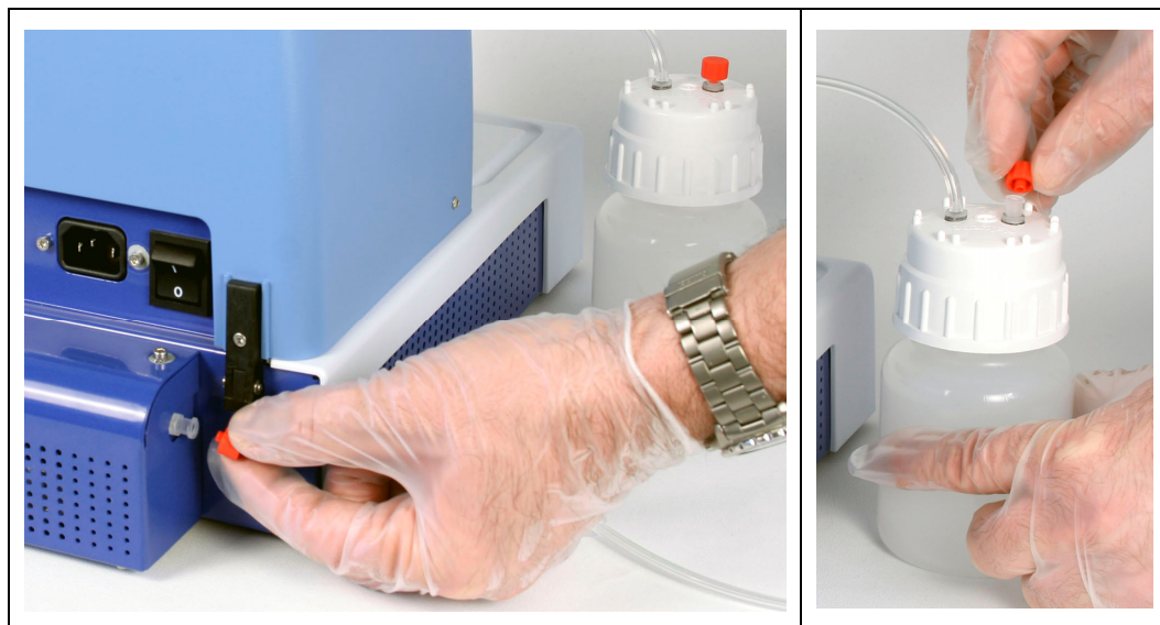
Figure 3–9. Removing the red luer plugs
