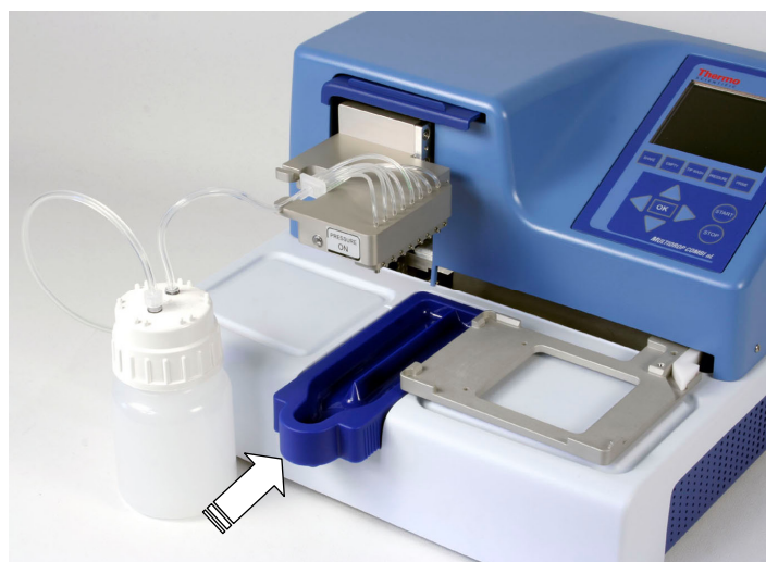
Figure 3–8. Inserting the priming vessel
